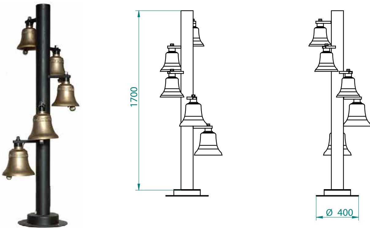
Ready to use small carillon bell set. This system is supplied completely assembled, wired and complete with eletrohammers (ELE3004001) and electrical power board, necessary for the connection of the unit to a master clock. Made up of 5 bells of "carillon" style in perfect musical chord, this product has been designed for small installations (roadside decorations, installation on roundabouts, as a compliment to advertising panels) where a competitive price is required.
